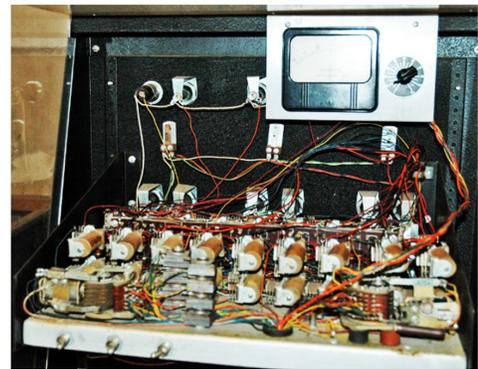
General Electric engineers here. Yola works in the Cathode Ray Tube Department, Bldg. 6. The tic-tac-toe machine was created by GE engineers Bert Liner, Bob Thor and Bob Hill.” The machine was truly a marvel of design – since its’ logic basically consisted of a number of hardwired latching and stepping relays. By the way, Jeff Houck-N2LYR now has this unit and is trying to get it functioning again.
