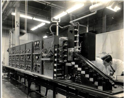
performance characteristics. A young engineer, Louis Agresti-W2OPF, was assigned the problem and developed a "Transistor Sorter" where transistors coming off the production line were run through an automatic tester that would drop each transistor into 1 of 8 different trays depending upon that unit's operating characteristics. The transistors in a particular tray were then marked with the part number appropriate for their characteristics.
