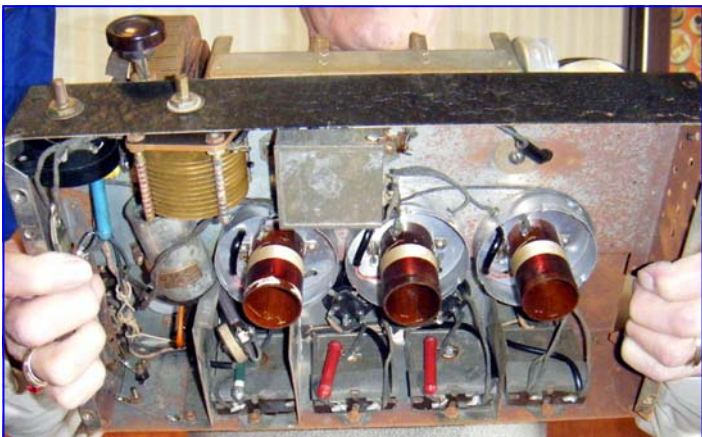
The American-Bosch radio, top and bottom chassis views.
